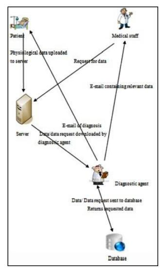
Fig. I. Proposed System architecture
